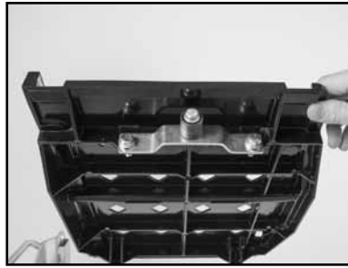
(E) Clean the Movable Cutting Table Roller Wheel and Frame Support
