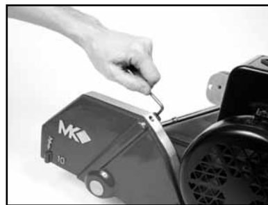
(G) Remove the Cooling Channel cover screws.
