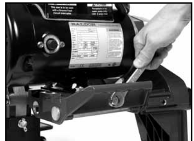
(F) Verify the Motor Adjustment Strap is tight.
