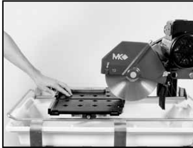
(B) Verify the Movable Cutting Table moves freely.
