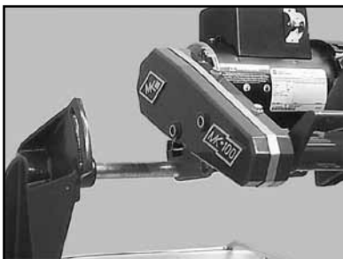
(G) Install the Cutting Head in rear Pivot Hole (Cutting Head Adjustment pg 25).
