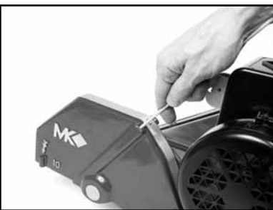
(H) Rod Cooling Channels and recheck flow.
