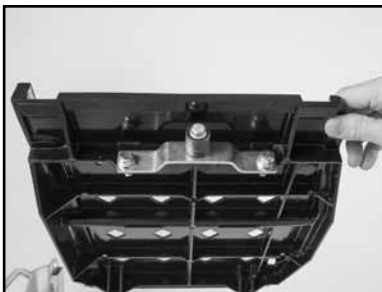
(D) Verify the Roller Wheel Assembly is tight and in good condition.
