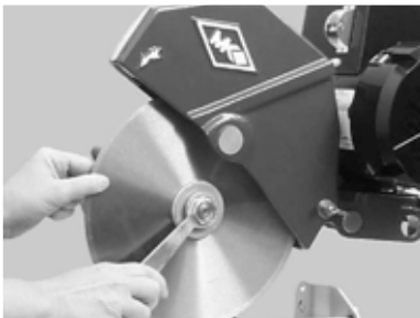
(A) Remove the Diamond Blade.
